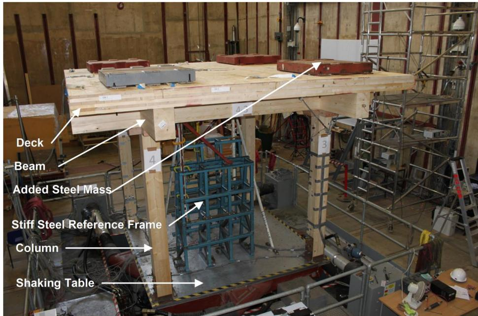
Figure 1: Typical testing layout of the BTC, based on [8]
