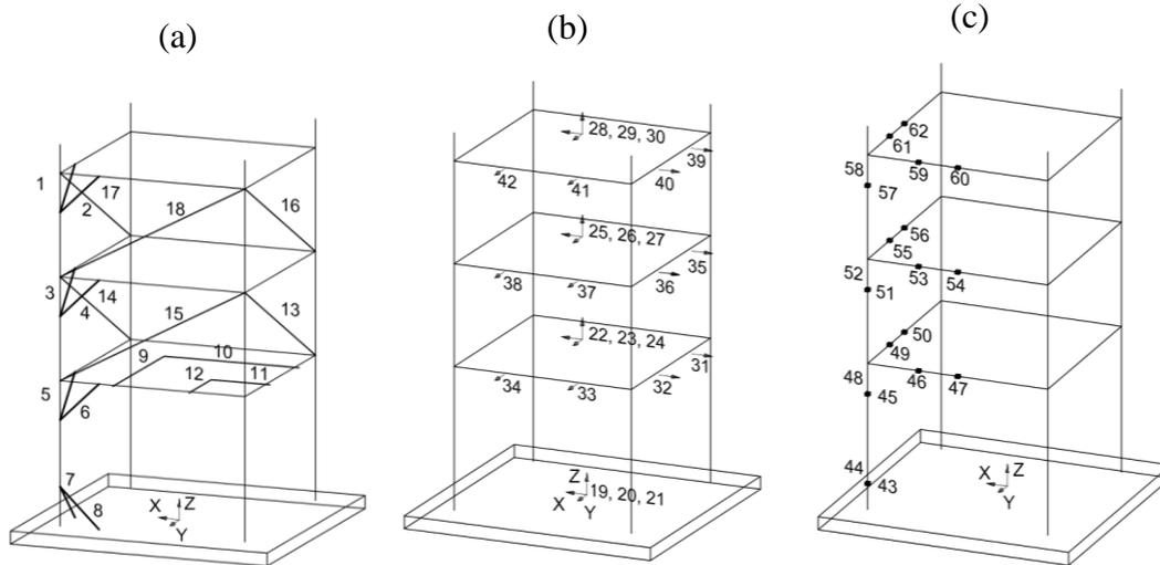
Figure 5: Schematic of the testing layout showing the location of (a) LVDT and potentiometers, (b) accelerometers and (c) strain gauges, based on [8]
