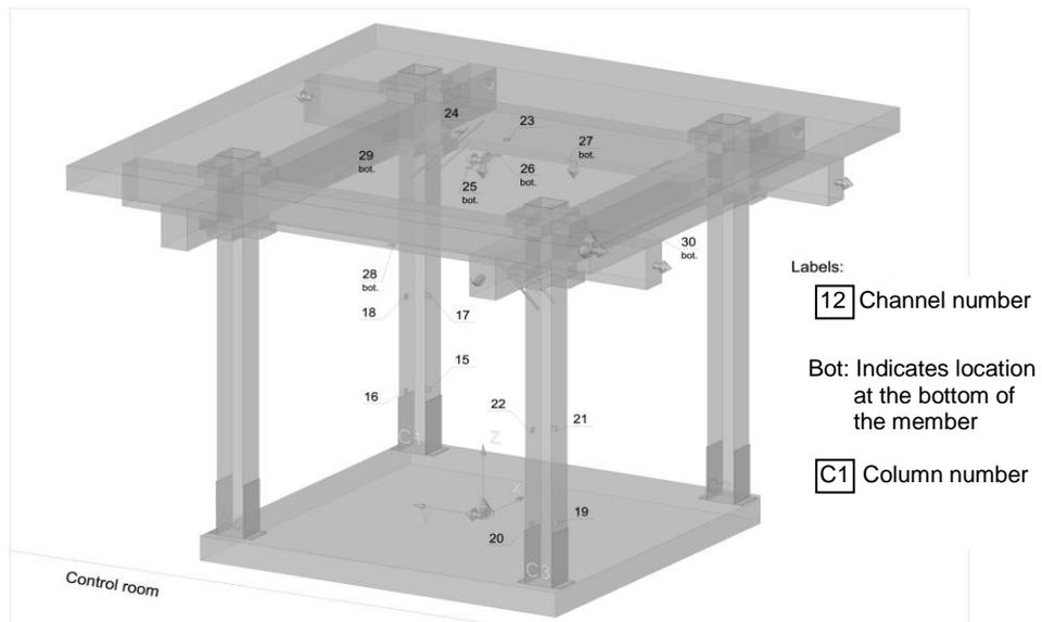
Figure 2: Locations of (a) accelerometers and (b) strain gauges, based on [8]
