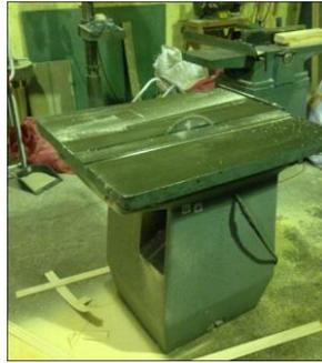
Figura 1: Sierra circular vertical fija
