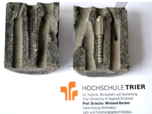
Figure 11: Opened specimen after testing
