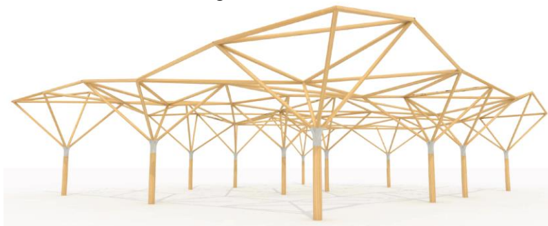
Figure 2: Spatial timber tree structure
