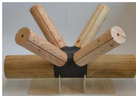
Figure 6: Finished CTA-joint with fitted trusses
