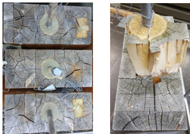
Figure 17: Service class 3 test specimen 365 days outdoor exposure (left), 720 days exposure after test (right)
