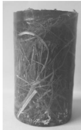
Figure 2: Guadua-polyester sample for compression tests
