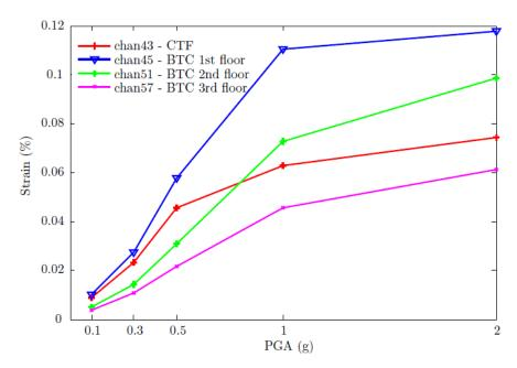
Figure 6: Stress increase on the different seismic tests at critical points of the structure, based on [9]
