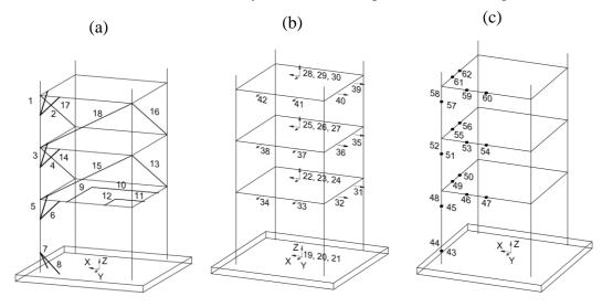
Figure 5: Schematic of the testing layout showing the location of (a) LVDT and potentiometers, (b) accelerometers and (c) strain gauges, based on [8]
