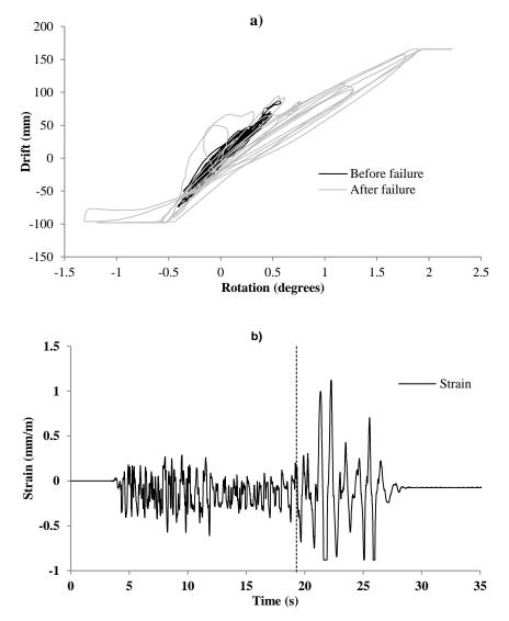
Figure 3: (a) Rotations versus drifts, and (b) strains in the one-storey frame during the third seismic test (1.43g PGA), based on [8]
