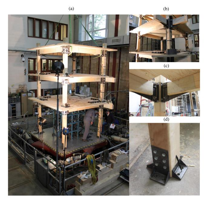
Figure 4: (a) scaled three-storey frame ready for testing, (b) detail of added steel masses, (c) detail of the BTC connection, (d) detail of the CTF connection
