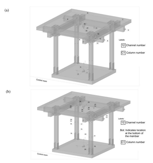
Figure 2: Locations of (a) accelerometers and (b) strain gauges, based on [8]
