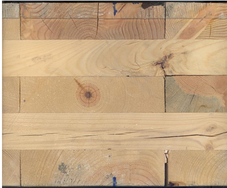
Figure 7: Checking, gap widening, material defect, and delamination in edge condition Specimen A, day 42
