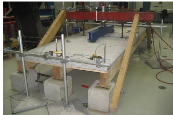
Figure 8: Experimental set-up of tested TCC ceilings
